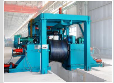
Double Drum Uncoiler for tube sizes of > \phi 165\text{mm}
